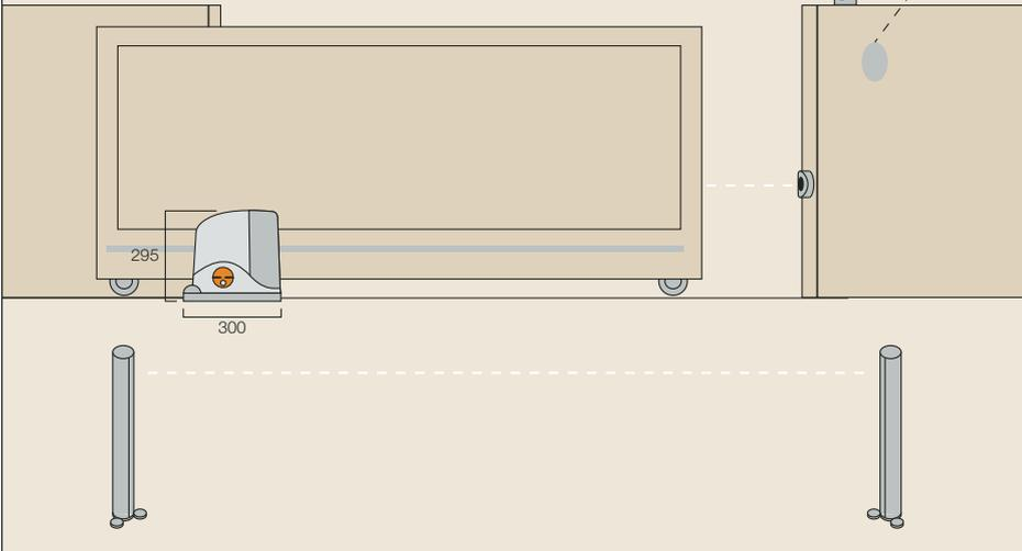
**1** The gear motor must be secured to a concrete base using the foundation plate
